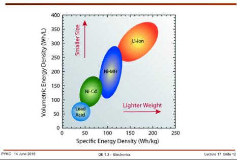
This plot shows how the four popular types of batteries vary in weight and size for a given
