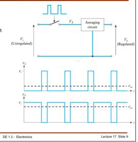
Even after using the full-wave rectifier circuit and the averaging capacitor, we still have to convert whatever DC voltage at the output to the desirable DC voltage. For that we use our old trusted PWM principle again.
